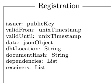
Fig. 4. A registration object including all possible fields which can be used to register a document via SPROOF.
