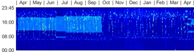
(a) Image construction from the normalized load profile with a color palette
