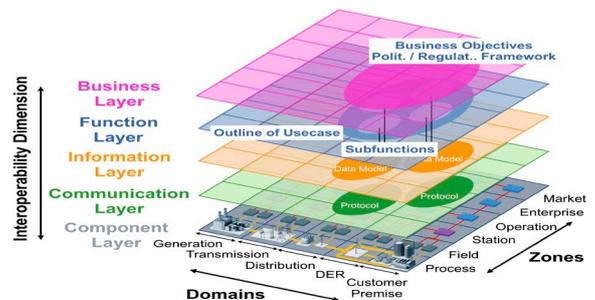
Fig. 1. Smart Grid Architecture Model [4].
