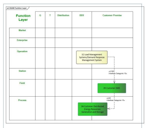
Figure 1 SGAM Mapping of the Interfaces
